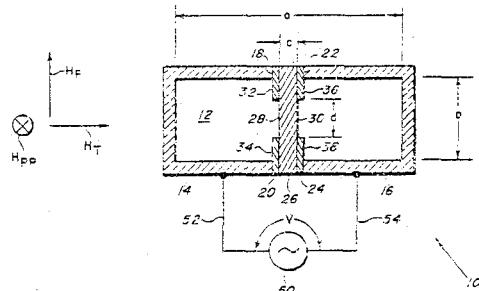
**Coaxial Dielectric Resonator Having Different Impedance Portions and Method of Manufacturing the Same**
